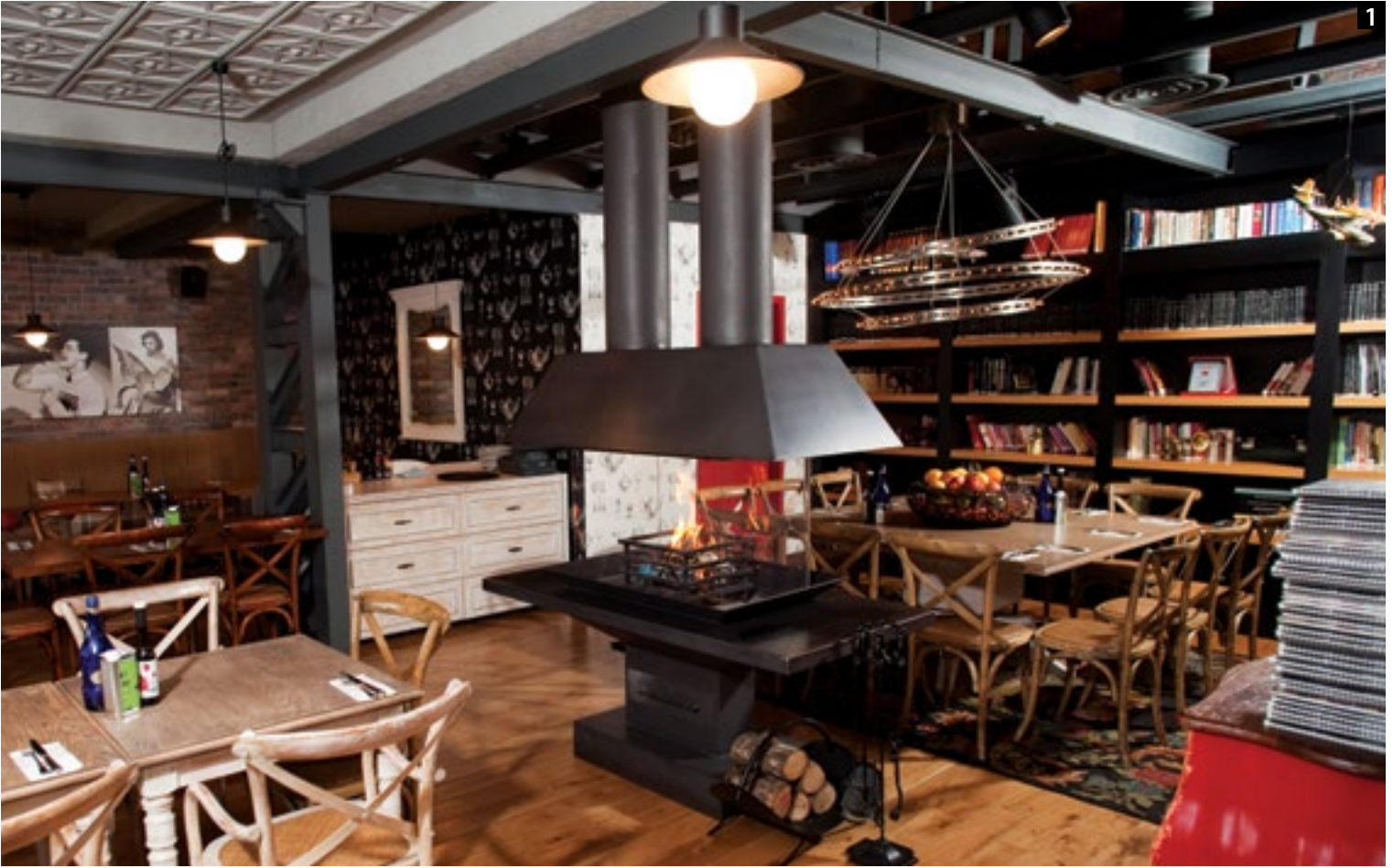
1 Steel Body and Chimney, Cast Iron Firebox, Custom Design Central Fireplace.
