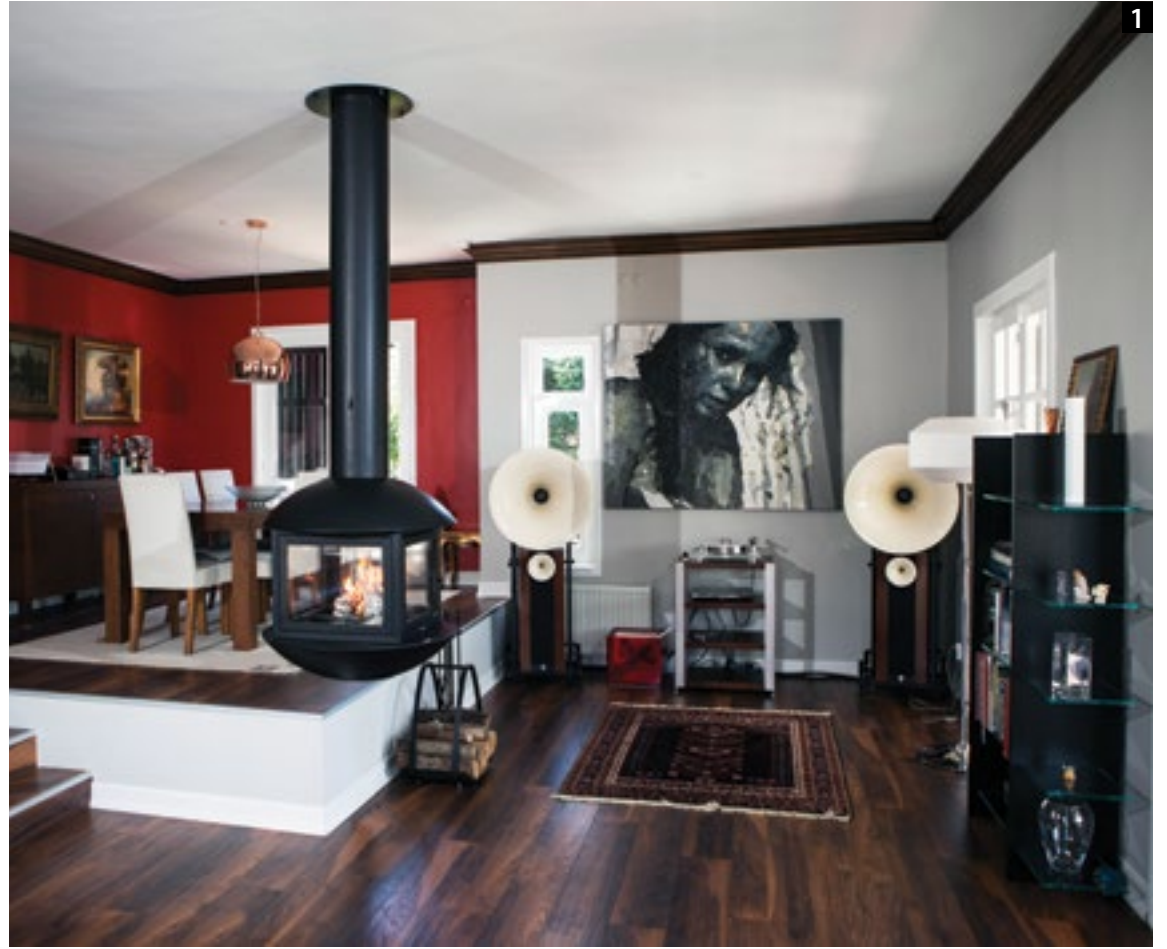
1 Four Side Glass, Steel Body and Chimney, Cast Iron Firebox, Suspended, 'Lantern' Model Central Fireplace.
