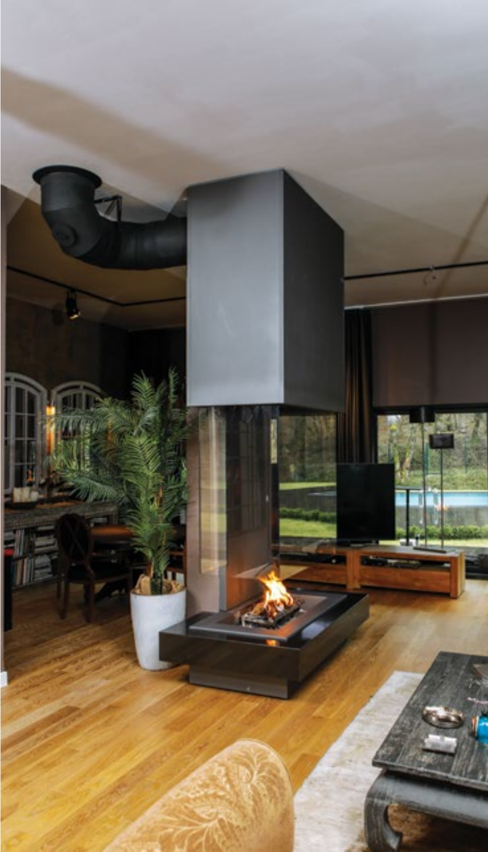
Vitro Ceramic Glass and Metal Chimney Hood; Cast Iron Firebox, 'Absolute Black' Granite Hearth, Custom Design Central Fireplace.
